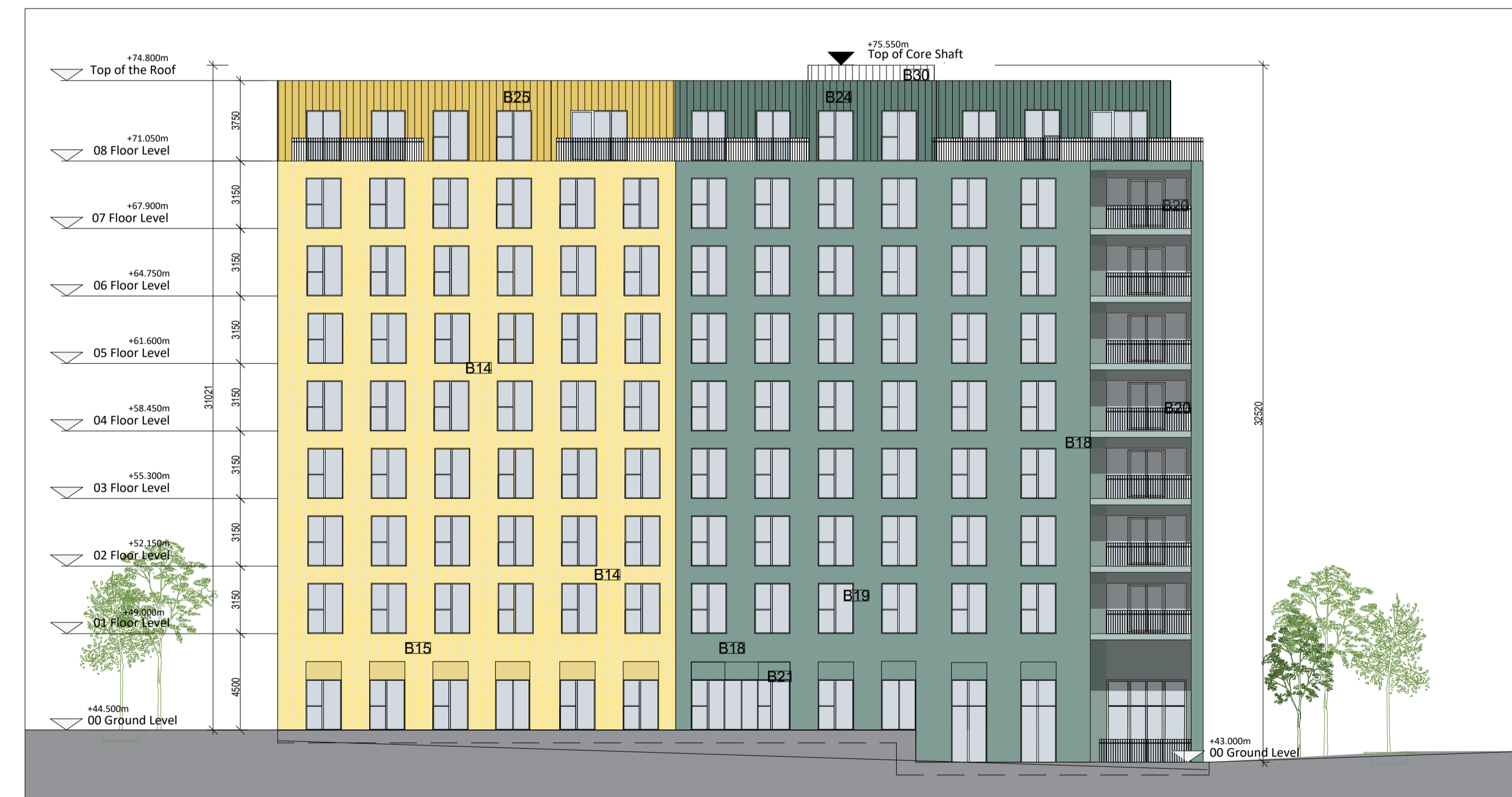
BLOCK 6 EAST ELEVATION 1:200@A1
