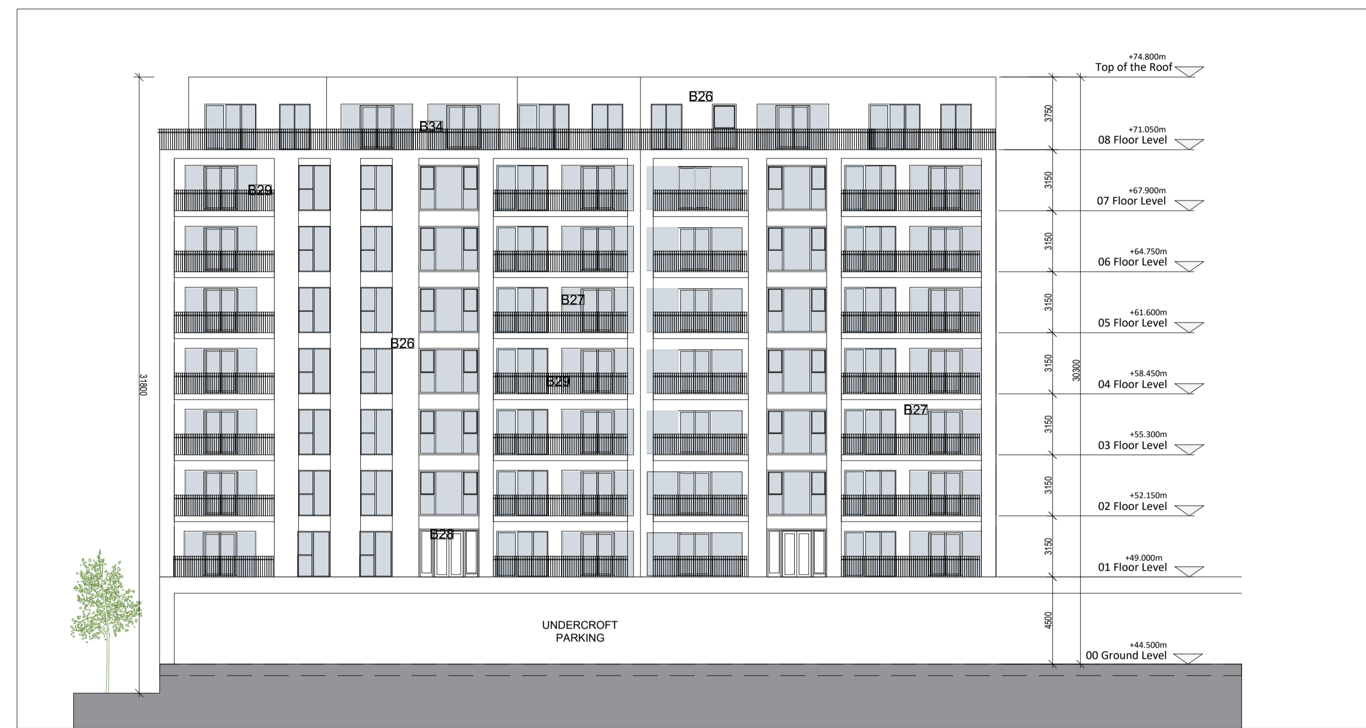
BLOCK 6 WEST ELEVATION 1:200@A1
